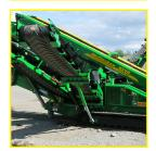
Conveyor Hydraulic folding 4th conveyor positioning allows for multiple height and angle options.
