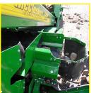
Cross Conveyor Cross conveyor replaces conventional chute and eliminates spillage and blockages.
